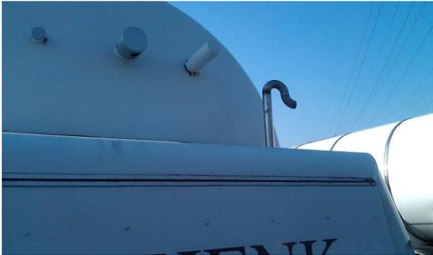
Tanker truck blow-off pipe
