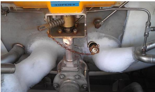
Ice formation on the pipes and hoses due to the transfer of the LNG
